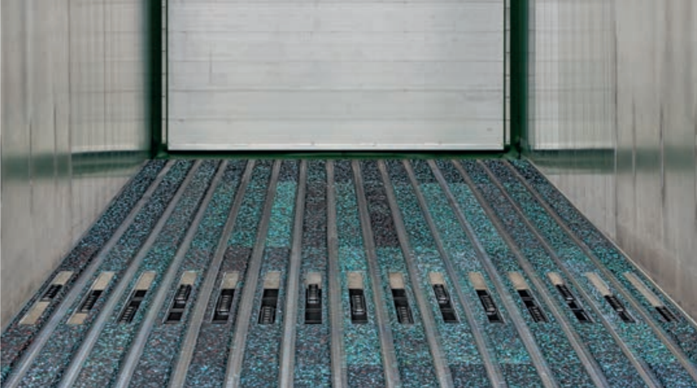
Only cut outs in subdeck for connecting drive-shoes to slat.
